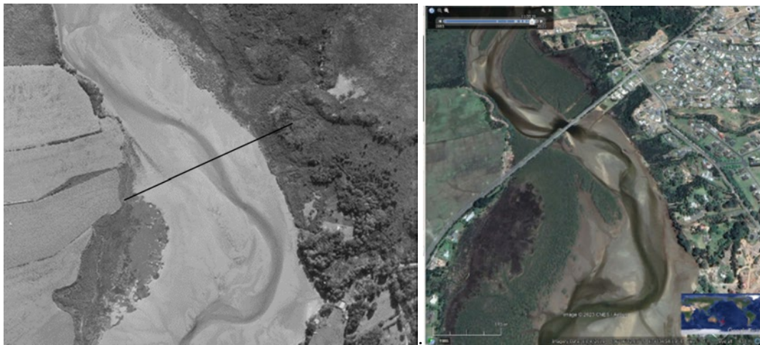
Figure 4-3. Comparison of channel morphology between pre-causeway situation in 1963 (left image) and post causeway situation in 2019 (right image) in area of the Molesworth Drive causeway. The black line on the left image shows the approximate line of the causeway. (Source: Images from Retrolens 1963 and Google 2019).
