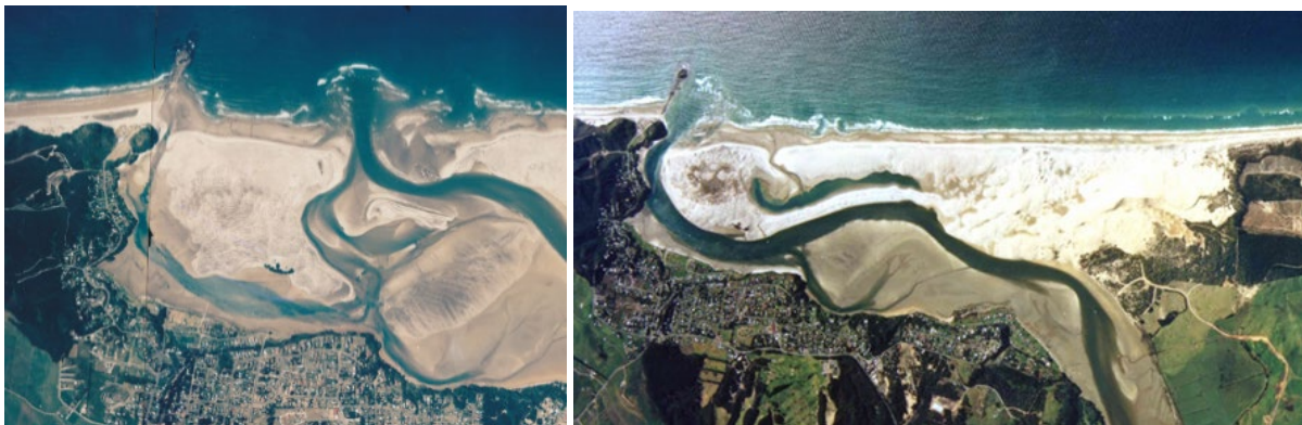
Figure 3-15. Left image shows situation in 1992 with northern entrance closed and southern entrance well established. Right image shows situation in August 1999 after engineering works. Northern entrance is now open. The bund wall can be seen in the vicinity of the neck and remnant ponds have a small channel connecting them to the sea (Source: A. La Bonté presentation).
