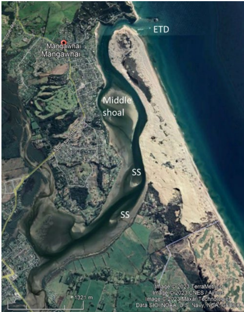
Figure 3-2. Features of the middle and lower harbour showing sandy shoals (SS) built by the incoming tide and the ebb tidal delta sand body (ETD). (Source Google Image 2003).
